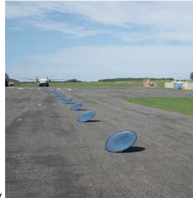
Point Source Array
