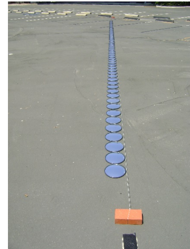
70 point facets create the linear target
