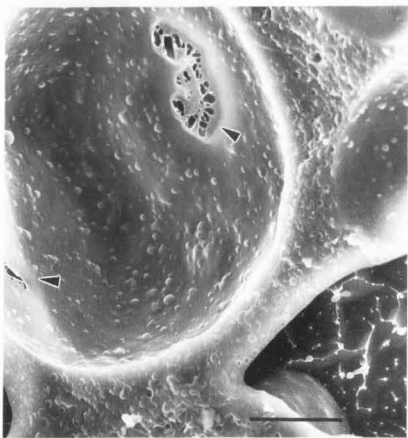
Figure 9 (top). Merged ice crystals (C) surrounded by the serum phase (S) in unstabilized ice cream after 24 weeks. Bar = 25 \mu m.
