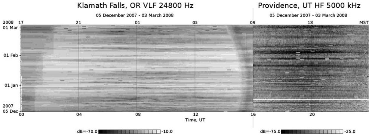
**Figure 8.** (left) Nighttime VLF propagation from NLK to KFO (0000–1600 UT) and (right) daytime HF propagation from WWV to PRV (1600–2400 UT) showing the relationship between VLF signal enhancement and HF absorption during the winter (5 December 2007 through 3 March 2008).
