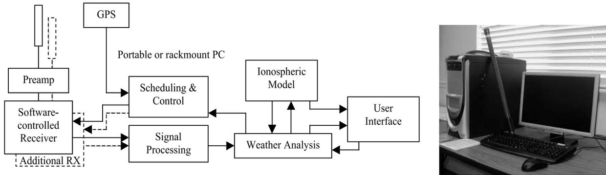
**Figure 1.** Conceptual sensor design including software block diagram and photo. The sensor consists of a Linux PC, a GPS receiver on top of the PC case, and a wideband active antenna leaning against the PC. The antennae are installed outdoors at roof level when deployed.
