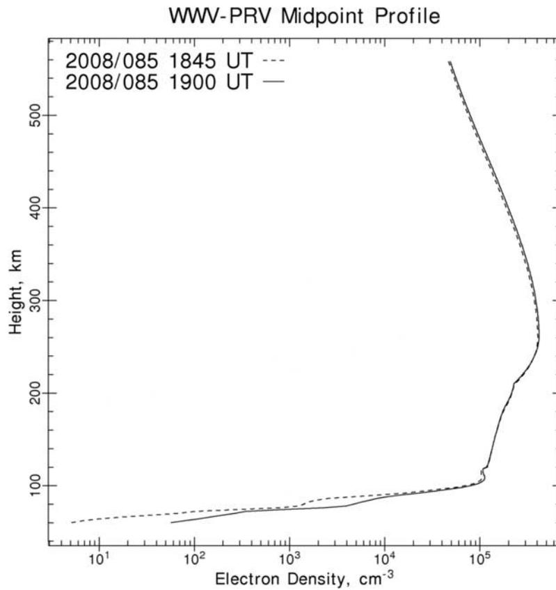
**Figure 11.** Ionospheric model of X-ray flare response. The electron density profile prior to the flare (dashed line) shows higher *D* region bottomside compared to the profile at the flare peak (solid line).
