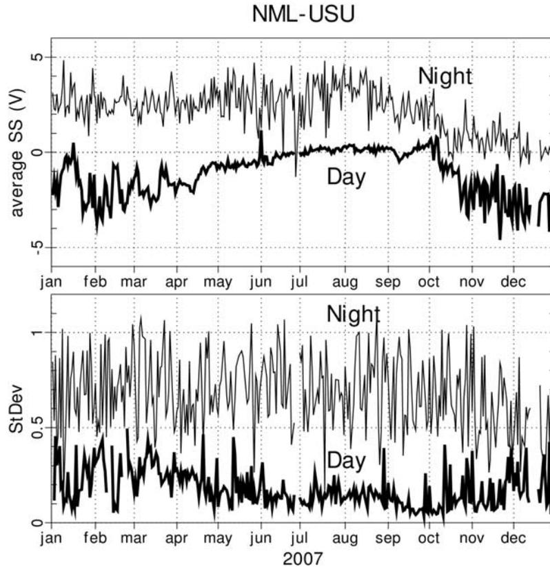
**Figure 5.** (top) Plot average signal strength for nighttime (0500–0900 UT) and daytime (2000–2200 UT). (bottom) Standard deviation of signal strength with time for daytime and nighttime signal during the same UT ranges. Daytime values are plotted with thick line.
