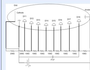
Fig. 6 - PMT schematic.
