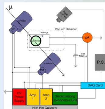
Fig. 10- Schematic of final setup to achieve coincidence between flares and muons.
