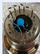
Fig. 7 - Wired PMT.
