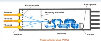
Fig. 8 - Diagram of PMT producing current.
