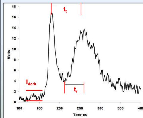
Fig. 5 - Example of counting pulses.
