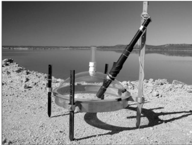
Figure 4—Assembled dome and probe/logger ready for use.
