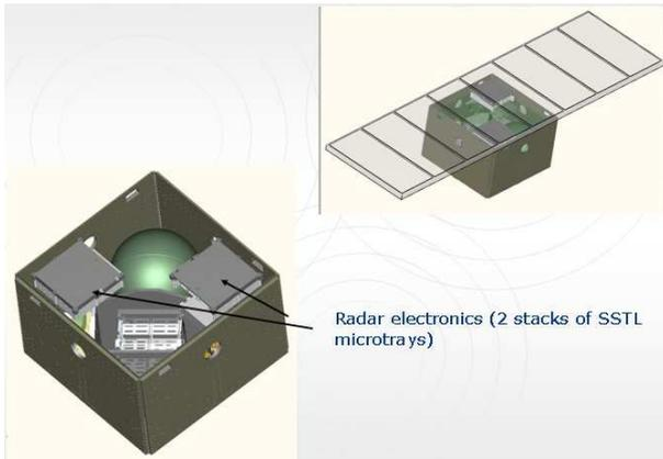
**Figure 7: DMC-SAR concept using SSTL-600 bus**
