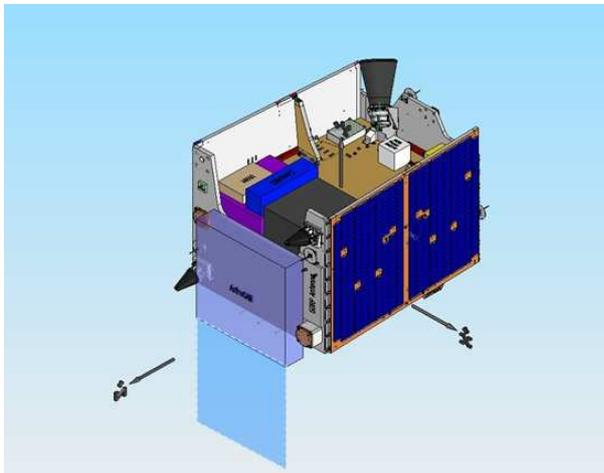
**Figure 8: DMC-SAR concept using SSTL-150 bus**
