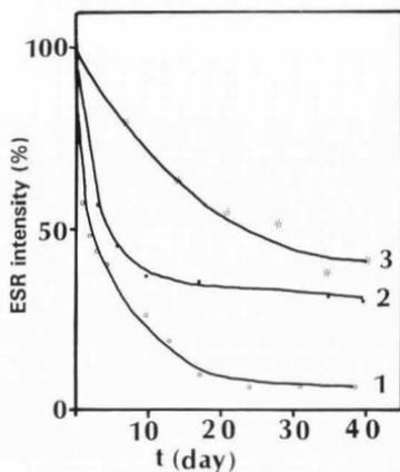
Fig. 4. The change of ESR intensity of samples of 36% protein content after 10 kGy irradiation in storage measurements under three different conditions: (1) at room temperature under normal conditions; (2) at room temperature in sealed ampoules; (3) at liquid nitrogen temperature in sealed ampoules.
