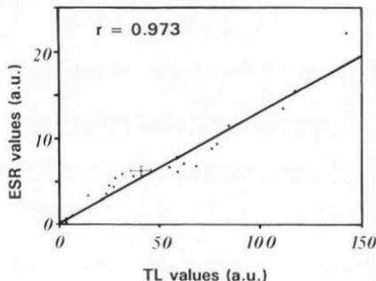
Fig. 7. Correlation between ESR and TL data of Tables 1 and 2. Correlation coefficient ( $r$ ) and error bars at one point for both measurements are given.
