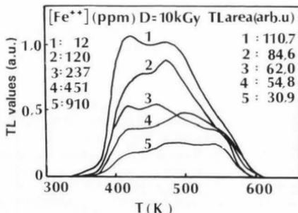
Fig. 6. TL curves at different ferrous ion concentrations for 10 kGy; a.u.: arbitrary units.
