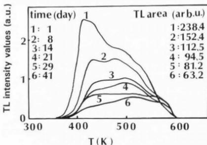
Fig. 5. TL curves and areas as a function of storage time at 36% protein content with 10 kGy absorbed ionizing  $\gamma$ -dose; a.u.: arbitrary units.
