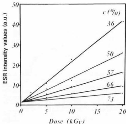
Fig. 2. ESR intensity as a function of absorbed ionizing  $\gamma$ -dose in the case of MPCP samples of different protein content; a.u.: arbitrary units.
