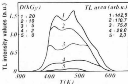
Fig. 3. TL curves and areas as a function of absorbed ionizing  $\gamma$ -dose at 36% protein content; a.u.: arbitrary units.
