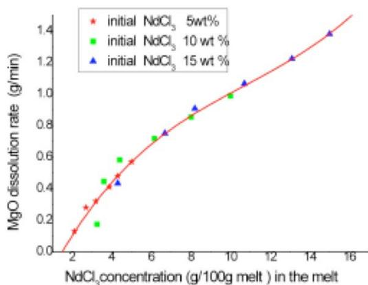
Figure 4—The relationship between the dissolution rate of MgO and NdCl<sub>3</sub> concentration.
