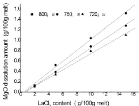
**Figure 8**—The effect of LaCl<sub>3</sub> content on the solubility of MgO (g/100 g melt).
