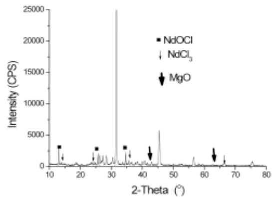
Figure 6—XRD patterns for NaCl:KCl:MgCl<sub>2</sub>:NdCl<sub>3</sub> (5:2:2:1 weight ratio) melts after dissolution of MgO.
