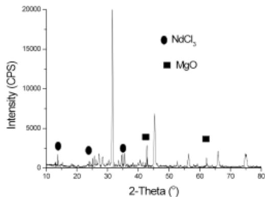
Figure 5—XRD patterns for a NaCl-KCl-MgCl<sub>2</sub>-NdCl<sub>3</sub> (5:2:2:1 weight ratio) melt with MgO melts before dissolution.
