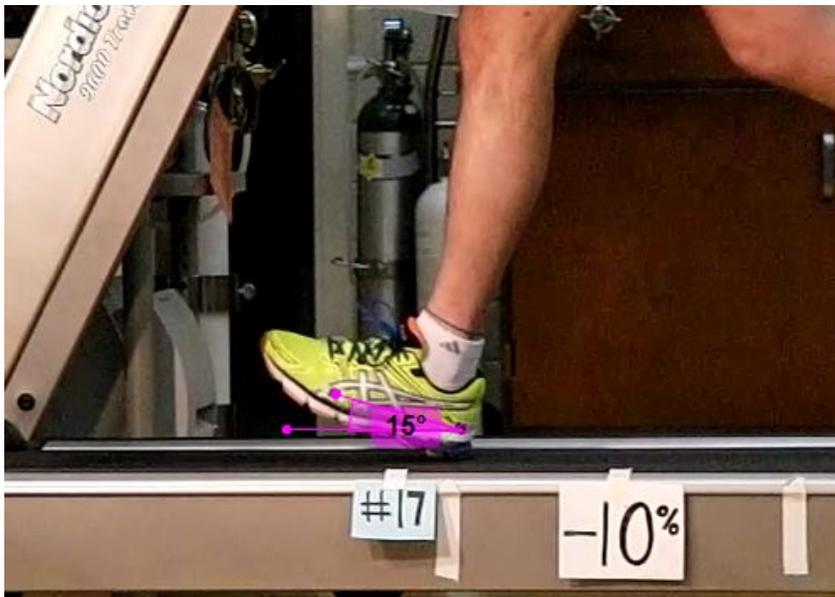
**FIGURE 1.** The foot angle at footstrike measured using the Kinovea angle-tracking tool. This is during the -10% from preferred SR condition for participant #17.
