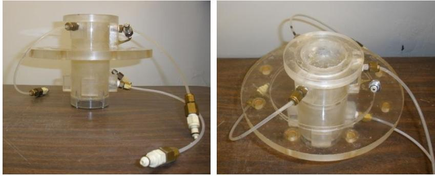
**Figure 2:** Soil container with ports for measuring pore pressures.
