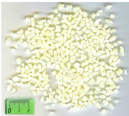
Fig. 1.1: Unprocessed acrylonitrile-butadiene-styrene thermoplastic. (Wikimedia Commons)
