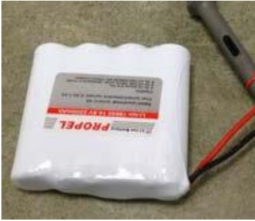
Figure 4: Li-ion battery pack.
