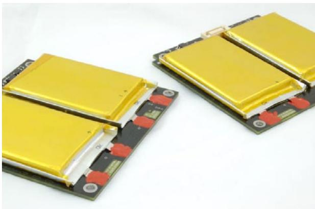
**Figure 4 Battery Daughter Boards; 1.25Ah at 8.2V**
