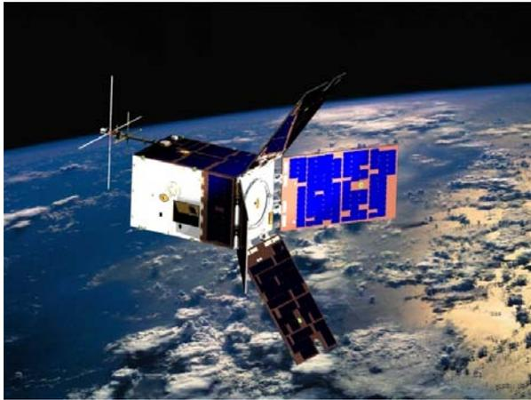
**Figure 1. Illustration of fully-deployed STPSat-1 SV on orbit, with CITRIS antenna on SV front, and circular standard separation adapter on back.**
