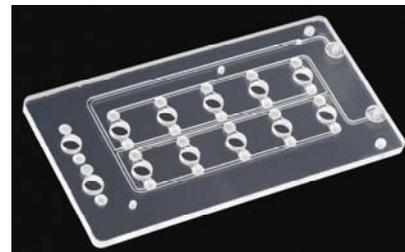
Figure 3: The GeneSat-1 Sample Well Plate
