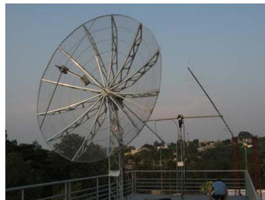
**Figure 17: 3m Dish and OSCAR Antenna**
