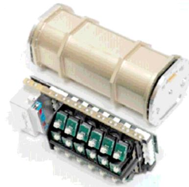
Figure 2: The GeneSat-1 Payload Module
