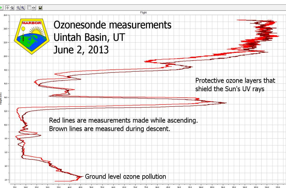
(above) Ozone data from the Ozonesonde. Line-of-sight tracking is required since the ozonesonde radio is weak. The data are then interpreted at the ground station from current levels to ppm measurement of ozone at specific altitudes. Other data are also in the downlink including position, temperature, and humidity.
