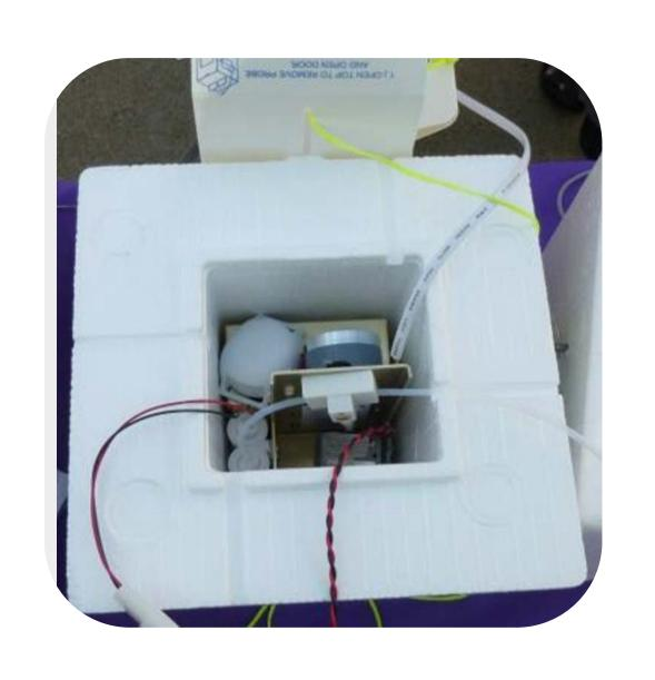
(left) The Ozonesonde, or ozone-detector, is like a small chemical laboratory. It has a small pump which takes in surrounding air and passes it through two chambers of chemicals. If ozone is present, the chemicals react, creating a potential cell that outputs direct current. The level of the current is transmitted to the ground station as data to be
