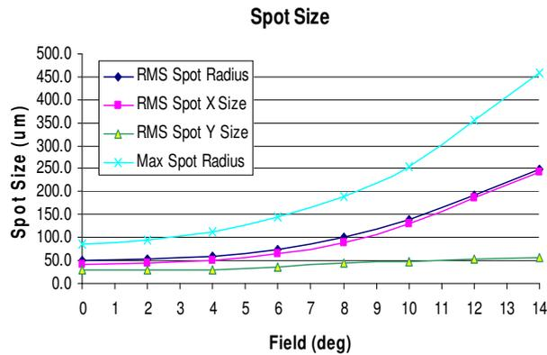
**Figure 4: Spot Size vs Angular Field**
