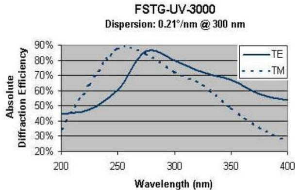
**Figure 6: Grating Diffraction Efficiency**
