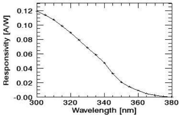
**Figure 7: Silicon Carbide Responsivity**
