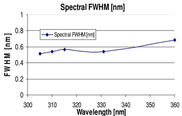
**Figure 3: Spectral Resolution (FWHM)**
