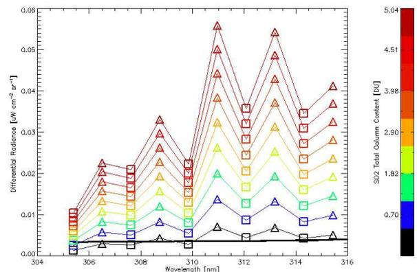
**Figure 9: Noise Equivalent Radiance Differential radiance of SO<sub>2</sub> laden w.r.t. Tropical Atmosphere**
