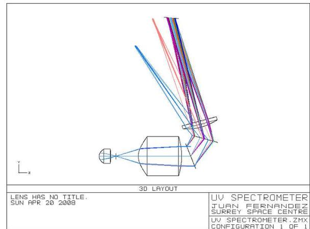
**Figure 2: Instrument Optical Layout**
