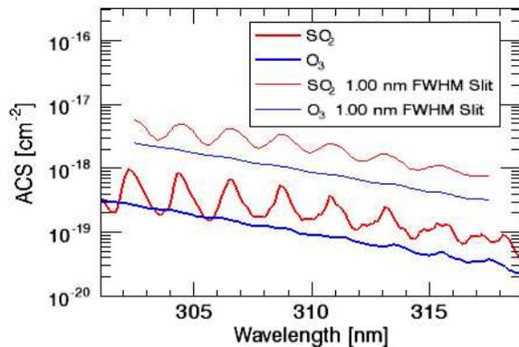
**Figure 5: Effect of Spectral Resolution of a 1-nm FWHM Slit Function.**
