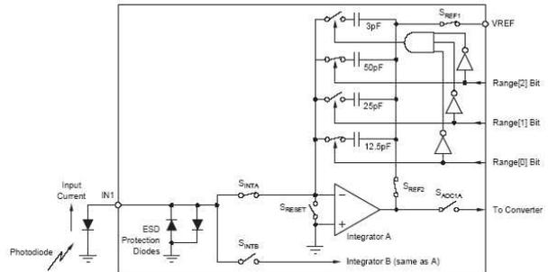
**Figure 8: Basic integration configuration**
