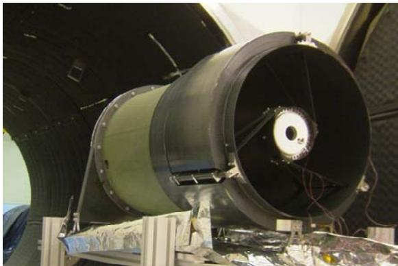
**Figure 3: RALCam-4 Structural Engineering Model in the Thermal-Vacuum Chamber**
