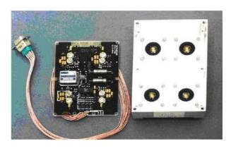
Figure 1 Ozone Mapping Detector (OMAD)
