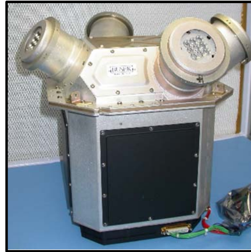
Figure 2: NASA ST7 Cluster of Four (4) Independently Operated Colloid Thrusters with 90 Days' Propellant Supply, Four (4) Power Processing Units (PPU), Field Emission Cathode, and Digital Control and Interface Unit (DCIU)
