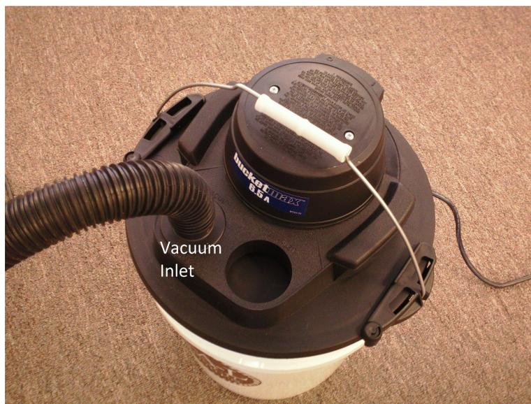
Fig. 2.13: Shop vacuum used as the pump for the plenum.
