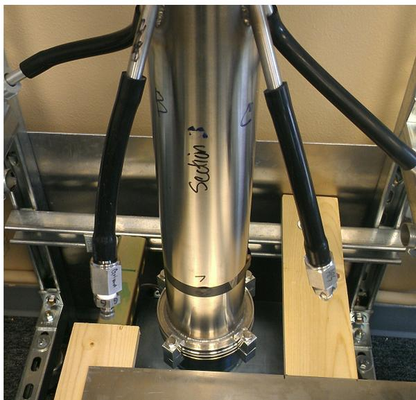
Fig. 3.15: Conductive tubing connections from the sampling ports to the instruments.
