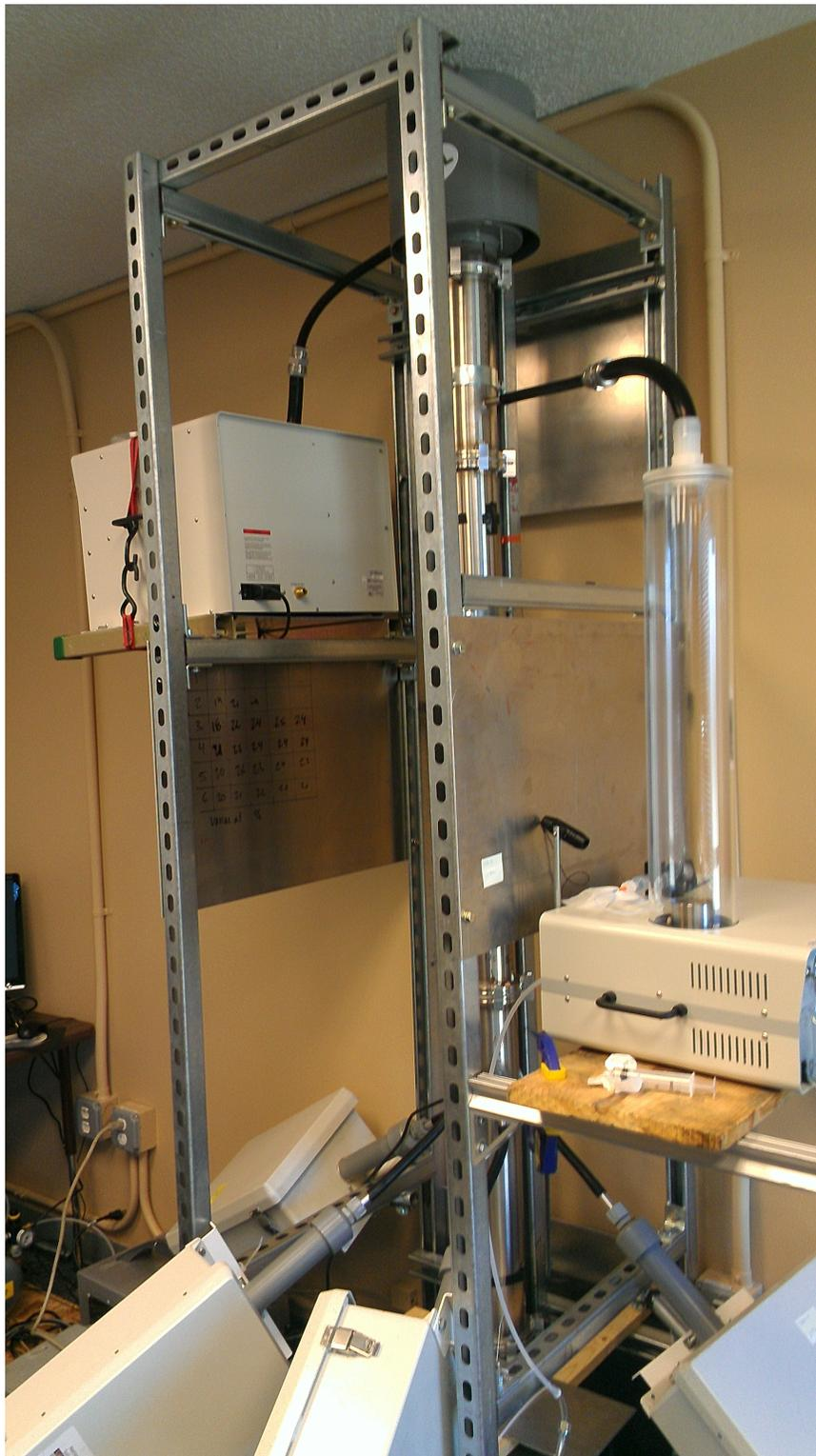
Fig. 3.17: Conductive tubing connections from the VOAG to the plenum.
