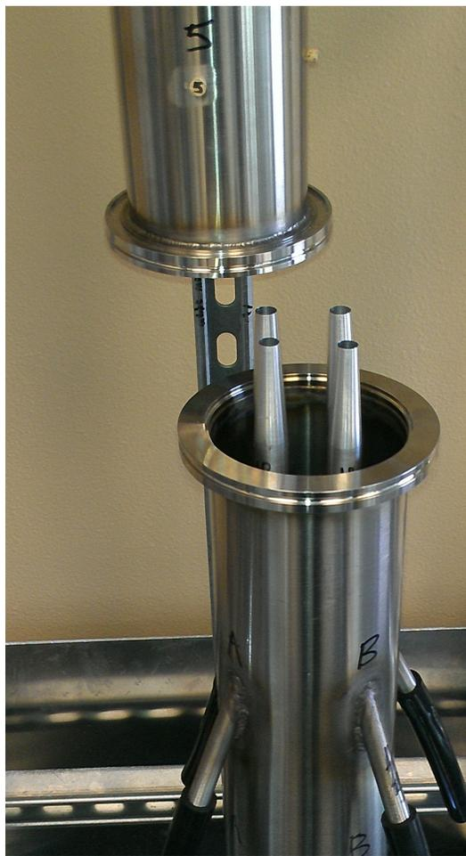
Fig. 5.7: Nozzles on section 2 of the plenum.
