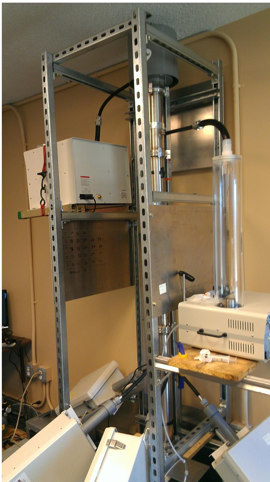
Fig. 5.4: Completed system with aerosol generators and instruments added.
