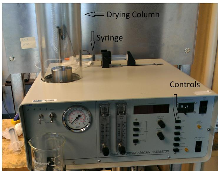
Fig. 1.11: Vibrating Orifice Aerosol Generator (VOAG), TSI Inc.
