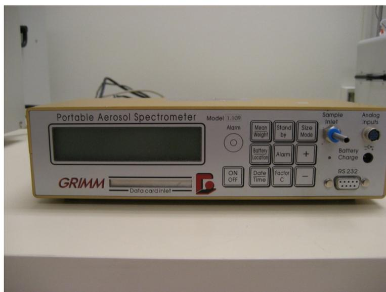
Fig. 1.5: Portable Aerosol Spectrometer 1.109, Grimm.
