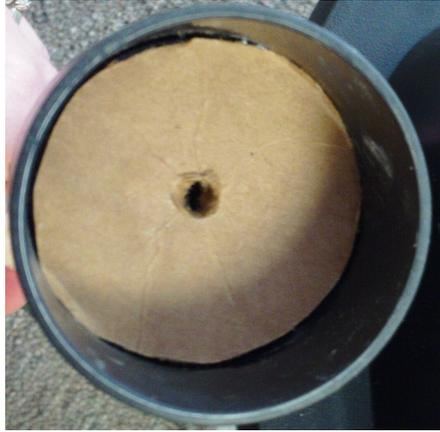
Fig. 2.14: Cardboard throttle plate to restrict the flow on the vacuum system.
