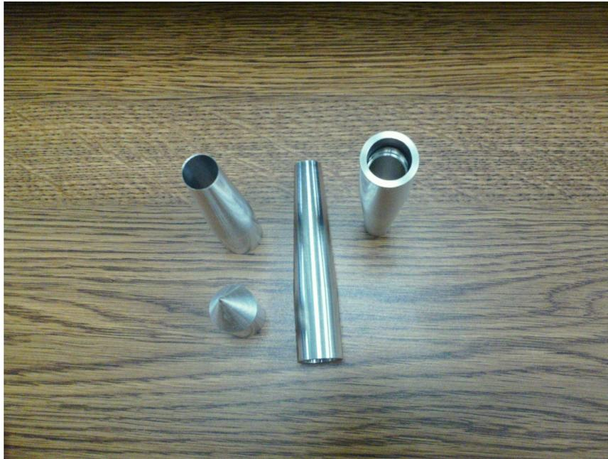
Fig. 2.9: Plenum nozzles for various flow rates.
