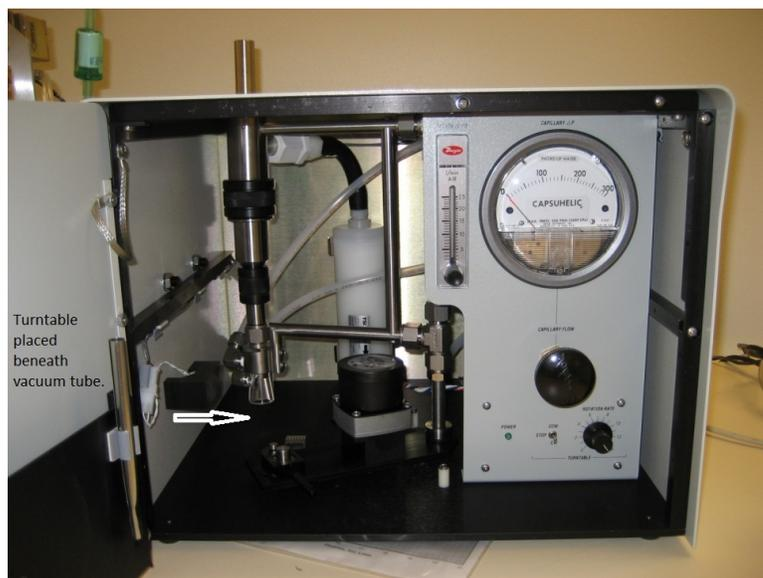
Fig. 1.9: Picture of internal pieces of the Small-Scale Powder Disperser (SSPD), TSI Inc.
