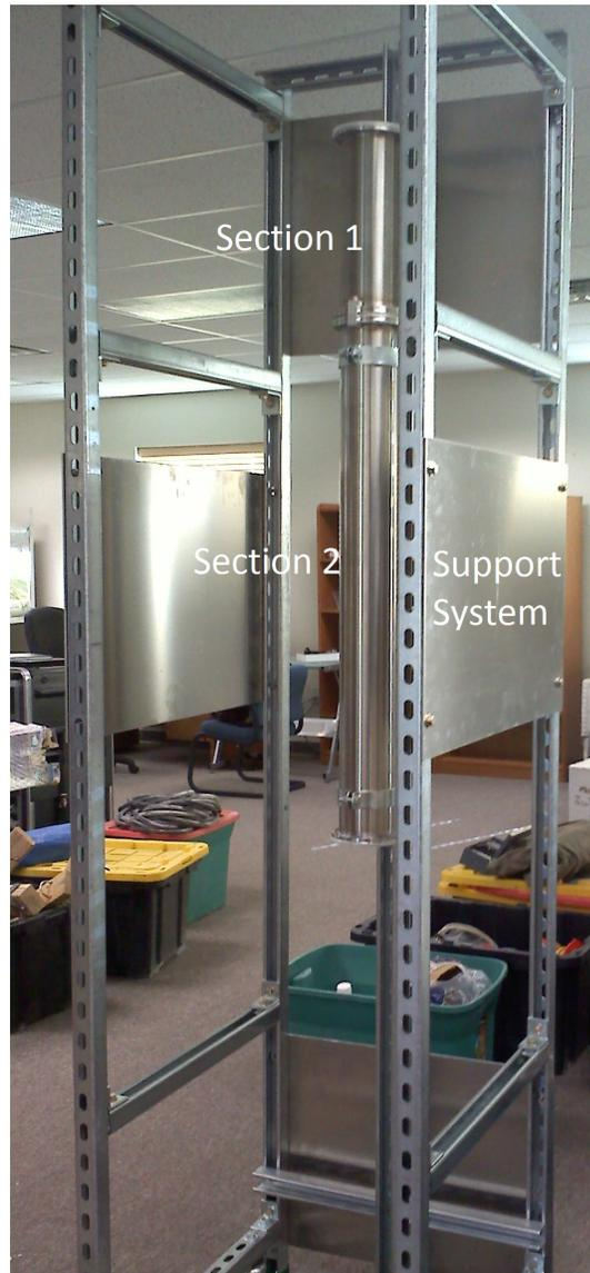
Fig. 2.15: Structural support for the calibration system.
