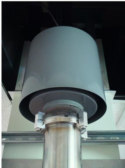
Fig. 2.7: A picture of the top filter with new flange as attached to the plenum.
