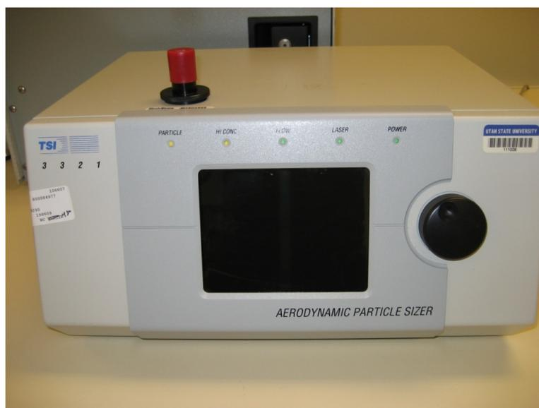
Fig. 1.3: Aerosol Particle Sizer, TSI Inc.
