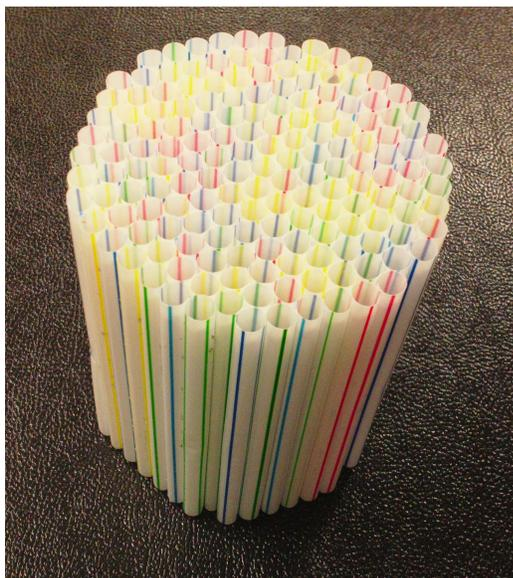
Fig. 3.6: Image of the final flow conditioner as placed in the system.
