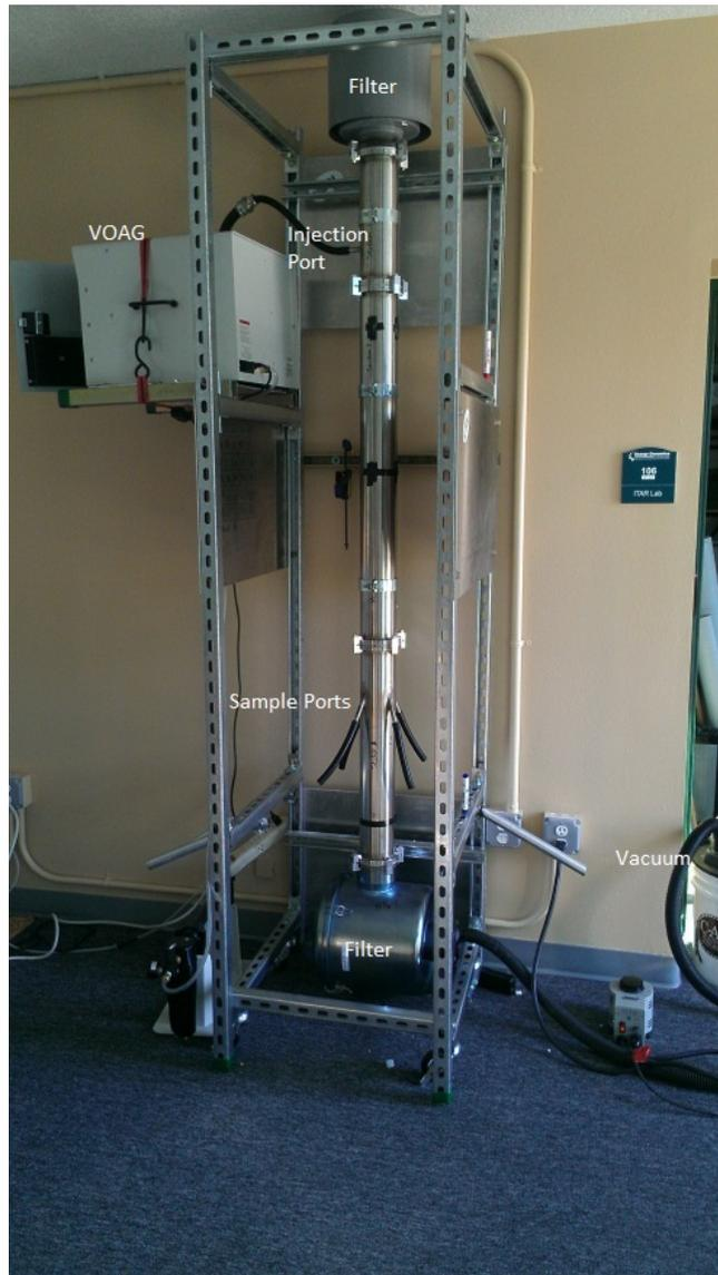
Fig. 2.16: Complete assembled calibration system.
