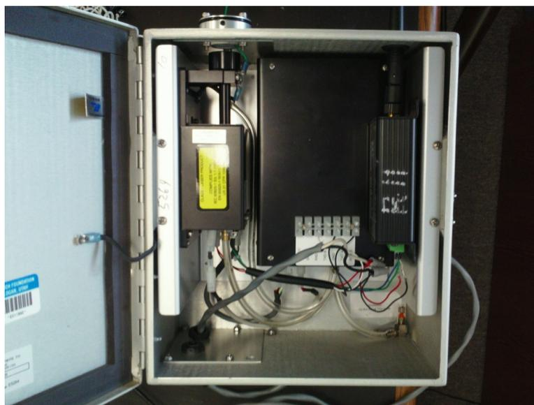
Fig. 1.7: Internal components of the Aerosol Profiler, Met One.
