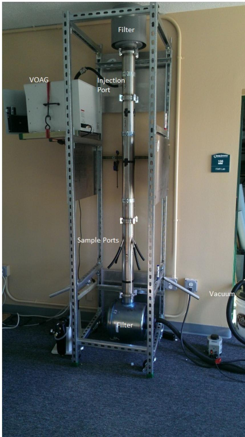
Fig. 5.3: Complete assembled calibration system.
