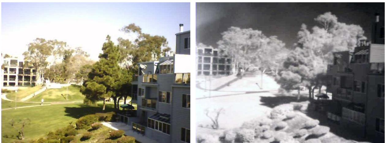
Figure 6. Two CMOS camera images of the same scene with (right) and without (left) a near-IR bandpass filter.
