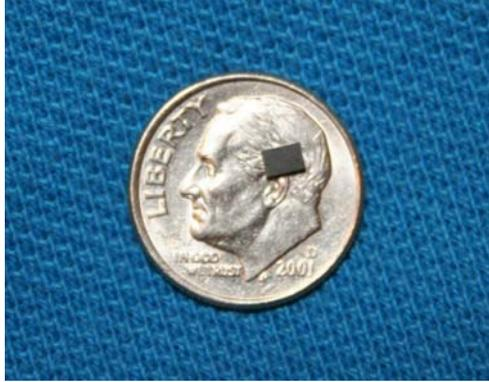
Figure 4. Photograph of a MicroChip PIC10F222 microprocessor on a U.S. dime. (A U.S. dime is ~18-mm in diameter)
