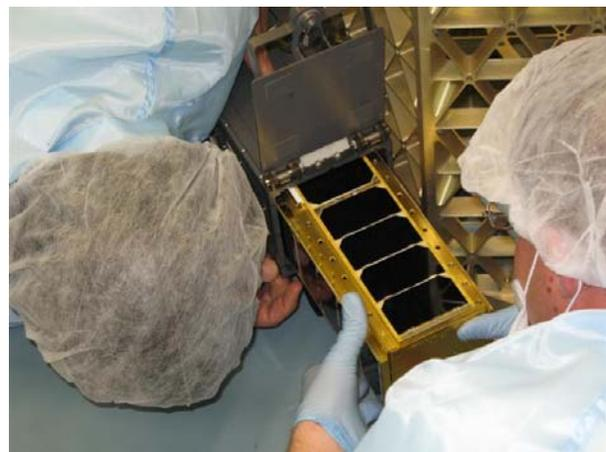
***Figure 7 NASA Ames Research Center's PRESat being integrated into a PPOD on the SPASS***
