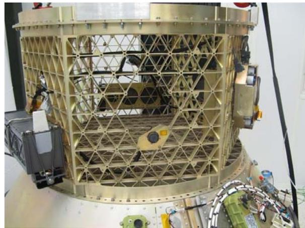
***Figure 6 SPASS integrated onto launch vehicle payload adapter and ready for primary payload integration***
