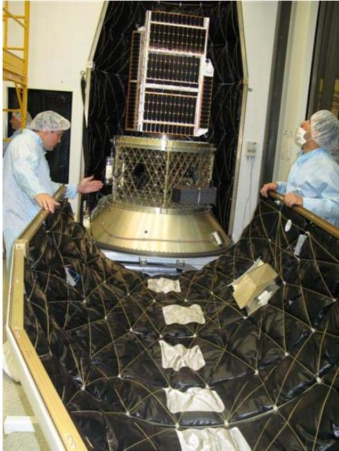
**Figure 8** *Jumpstart mission integrated payload stack ready for fairing encapsulation*
