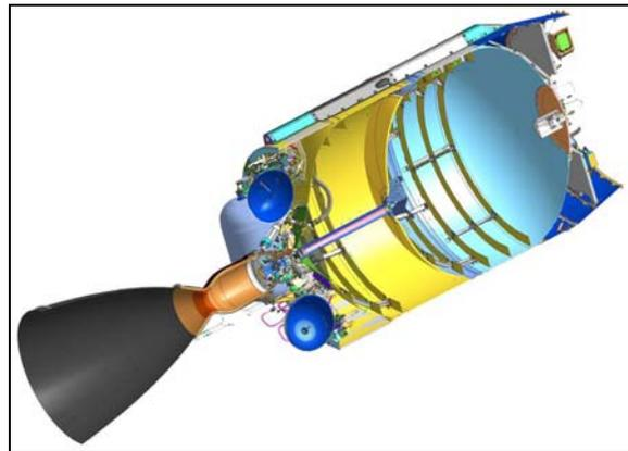
**Figure 3 Stage 2 cross section illustrating internal slosh baffles**
