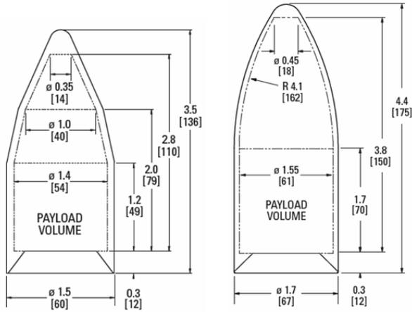
**Figure 4 Falcon 1 and Falcon 1e payload fairing dimensions**
