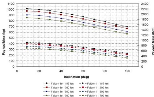
**Figure 5 Falcon 1 and Falcon 1e payload capability**
