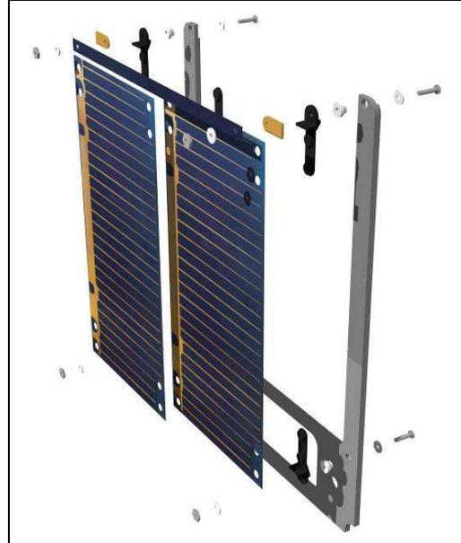
**Figure 3: Thin Film Solar Cells**
