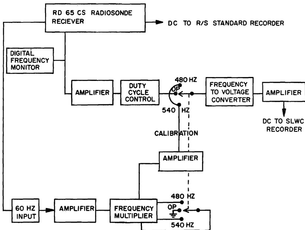
Fig. 3. Block diagram of modified rawinsonde receiver for obtaining SLWC data.
