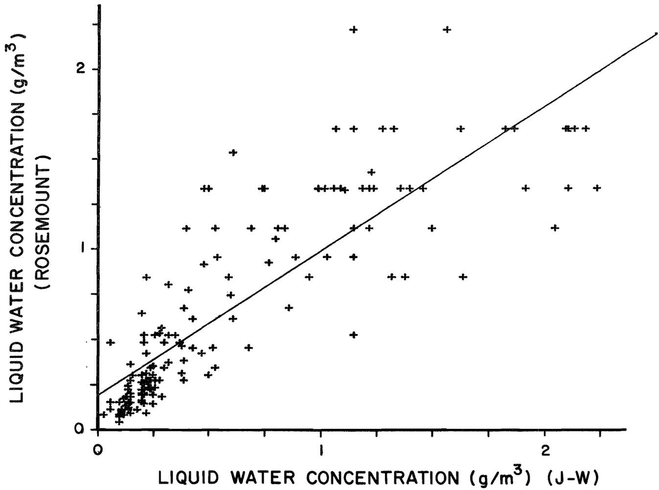
Fig. 13. Liquid water concentrations measured by Johnson-Williams and Rosemount devices for 6 events in FY78 and 79.
