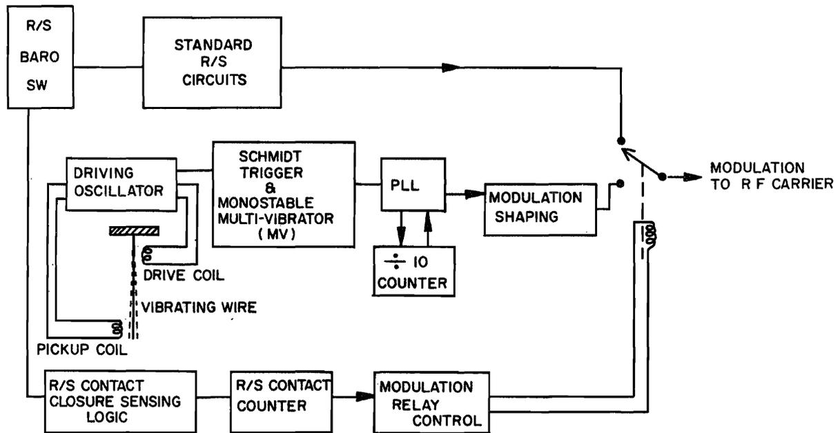
Fig. 2. Block diagram of modified rawinsonde for measurement of SLWC.
