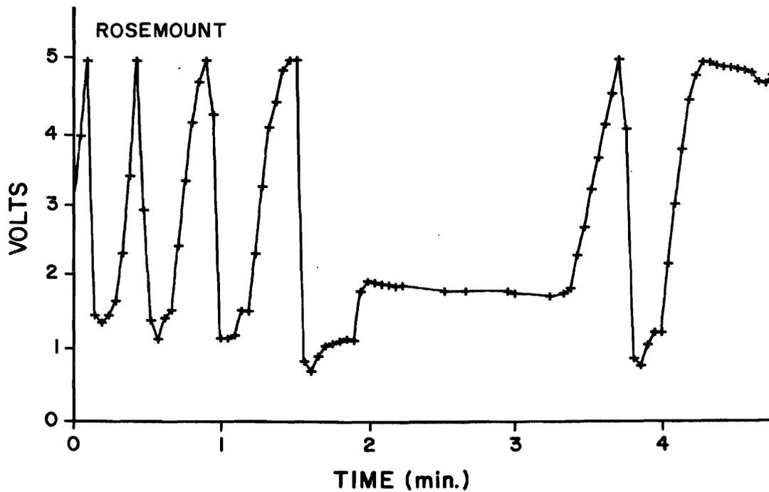
Fig. 10. Sample liquid water raw data for Johnson-Williams vs Rosemount devices with moderate concentration of liquid water.
