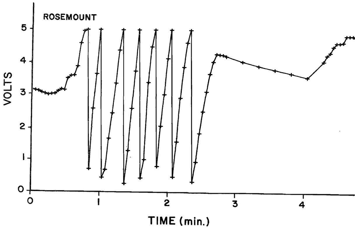
Fig. 12. Sample output of Rosemount device in and out of cloud.
