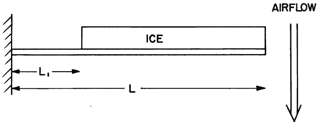
Fig. 1. Illustration of ice-loaded wire.
