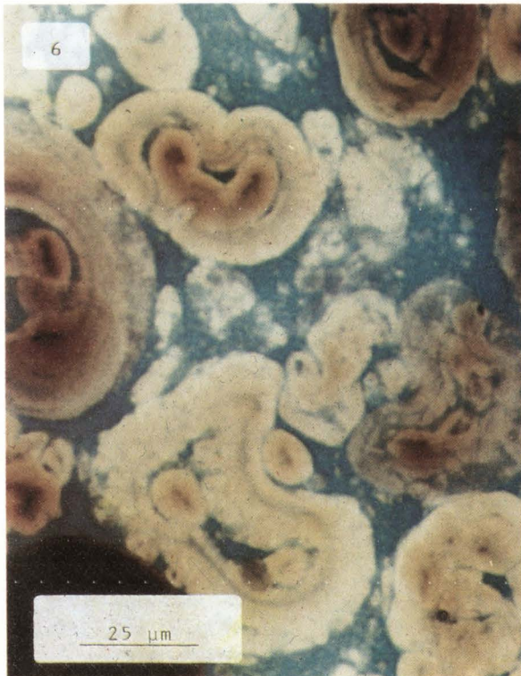
Figs. 4-6. Smears of 8% barley starch suspensions heated to 90 ( Fig. 4 ), 95 ( Fig. 5 ), and 95°C for 15 minutes ( Fig. 6 ).
