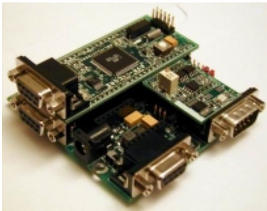
**Figure 9: SCU AVR-SAT Flight Computer**
