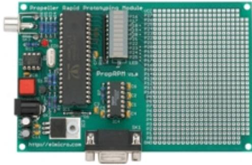
**Figure 7: Parallax Propeller Development Board**
