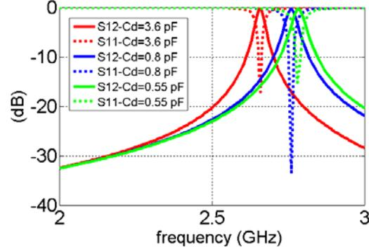
**Figure 3: S11 (reflection) and S12 (transmission) of single tuning block for various  $C_d$**
