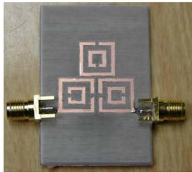
Figure 8: Fabricated third order tunable bandpass filter
