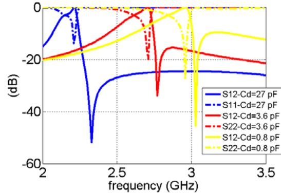
Figure 7: Simulation results of third order tunable bandpass filter various varactor capacitances
