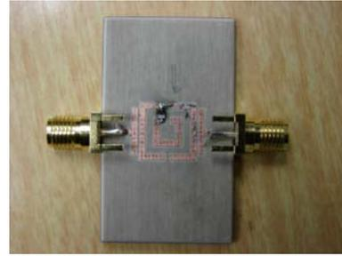
**Figure 4: Fabricated basic tuning block.**
