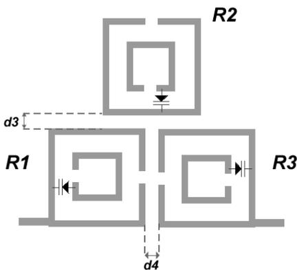
Figure 6: Schematic of the third order bandpass filter with single transmission zero located on the right side of passband.
