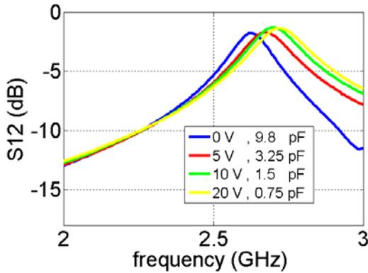
Figure 5: Measured S12 of single tuning block for various biasing voltages
