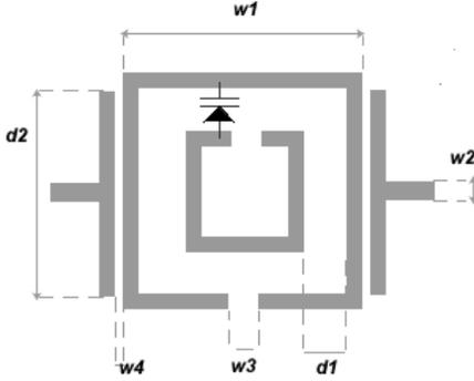
**Figure 1: Schematic of varactor loaded SRR tuning block. Metal regions are depicted in gray.  $w_1=10$ ,  $w_2=2.9$ ,  $w_3=1$ ,  $w_4=0.5$ ,  $w_5=8$ ,  $d_1=1.5$ ,  $d_2=8$ . All the dimensions are in mm**
