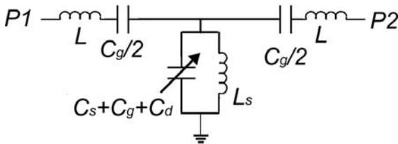
**Figure 2: Equivalent lumped element circuit model for single tuning block.**
