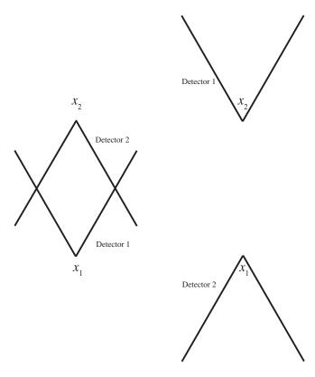
FIG. 1. The arrangement of the two BBO detectors described [17] and the arrangement actually analyzed when  $\gamma'_{12}$  is substituted for  $\gamma_{12}$ . Owing to its larger spatial extent, the system actually studied is much more sensitive to frequency than the system whose study was intended.
