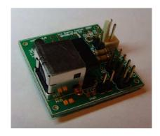
Fig. 2.3: OSIF i2c to USB board.
