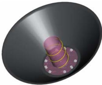
**Figure 9: Payload-side TT&C antenna (monofilar helix with conical shield; Ge-Kapton cover not shown).**
