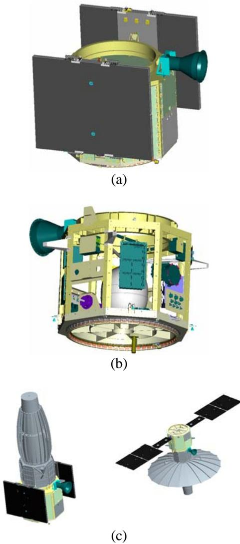
**Figure 5: Prototype ORS Spacecraft Configuration: (a) and (b) Spacecraft Bus Component Layout; (c) Space vehicle configuration, stowed and deployed**
