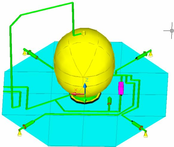
**Figure 7: Passive Thermal Design For Propulsion Subsystem Temperature Control**
