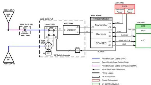
**Figure 8: RF System Block Diagram**
