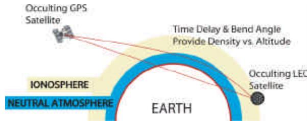
Figure 5: Geometry of GPS or GNSS RO
