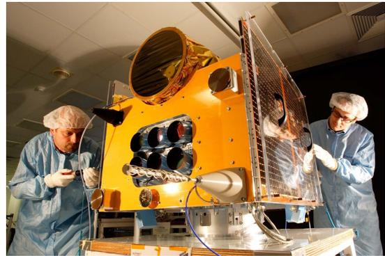
**Figure 3: Beijing-1, high resolution and wide swath 160kg class microsatellite**
