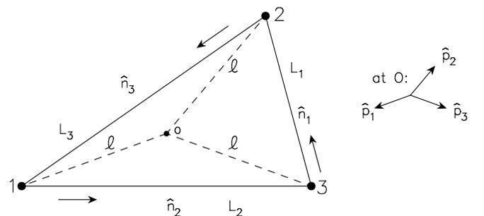
FIG. 1. Schematic LISA configuration. Each spacecraft is equidistant from point  $o$ , with unit vectors  $\hat{p}_i$  indicating directions to the three spacecraft. Unit vectors  $\hat{n}_i$  point between spacecraft pairs with the indicated orientation.
