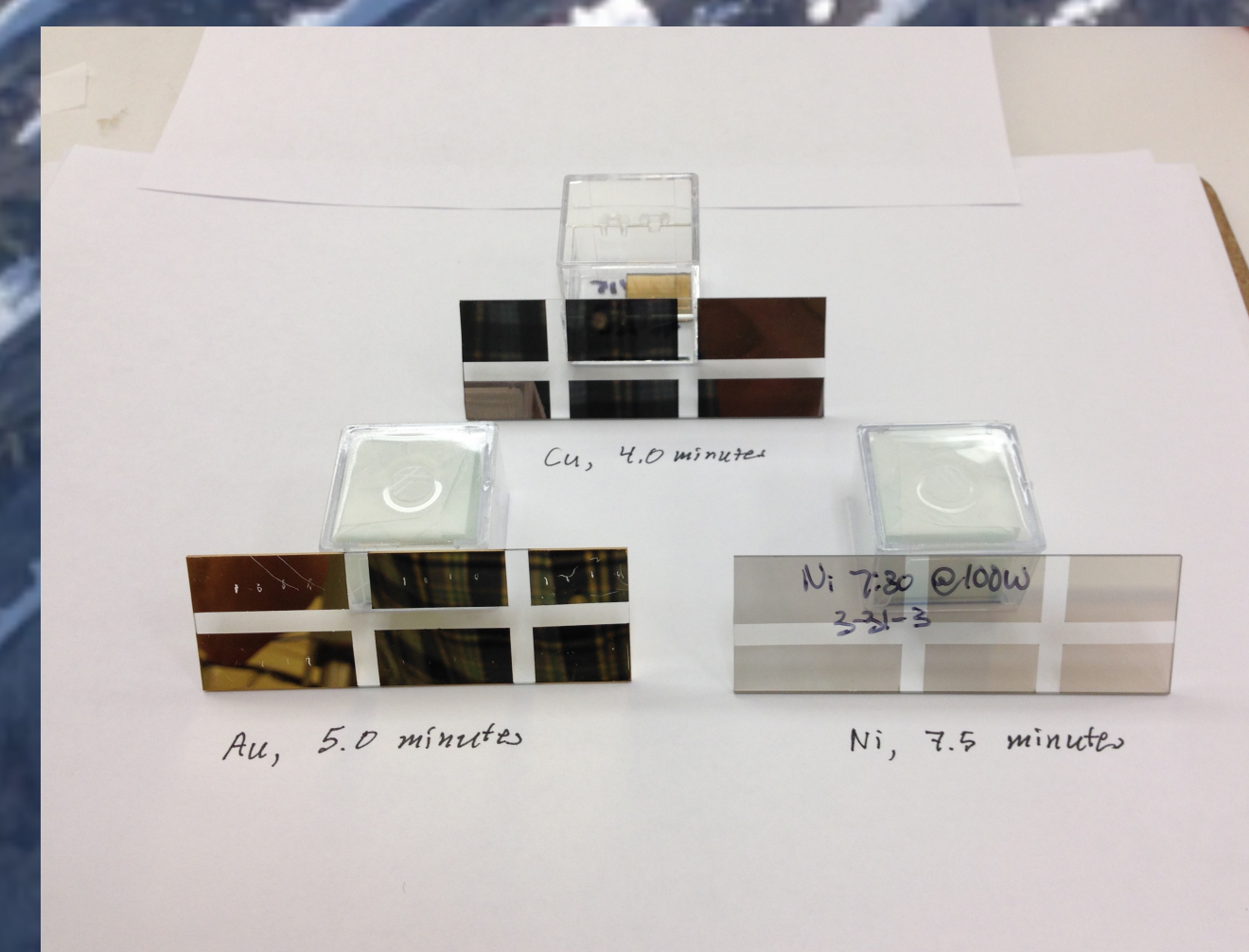
Samples of Au, Cu and Ni, produced on glass in panels, that aid in resistivity and profilometry measurements
