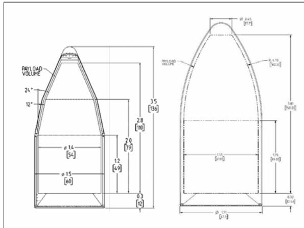
**Figure 4 – Falcon 1 and Falcon 1e payload fairing dimension comparison**
