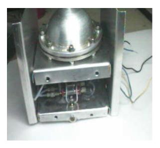
Figure 7: A Prototype Cubesat Propulsion Module Used for Thruster Hot Fire Tests.
