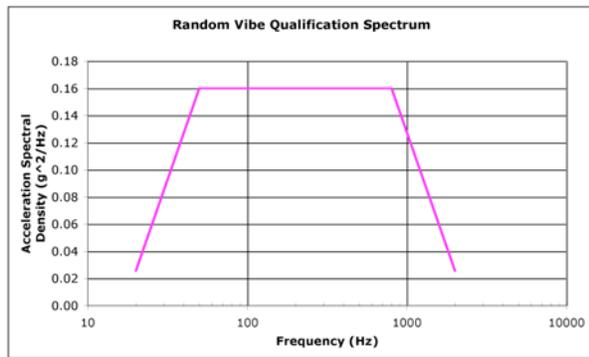
**Figure 6: Vibration Spectrum.**
