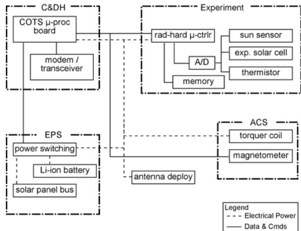
**Figure 7. Solar Cell Measurement System Block Diagram.**
