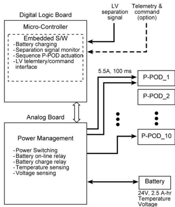
Figure 5: NPSCuL Block Diagram.
