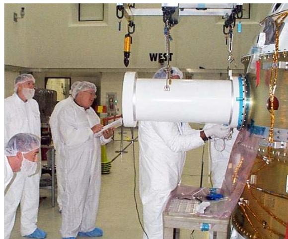
**Figure 1: NPSAT1 mass simulator installed on ESPA-ring on STP-1.**
