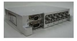
Figure 4-10: Communication Unit (BBM)
