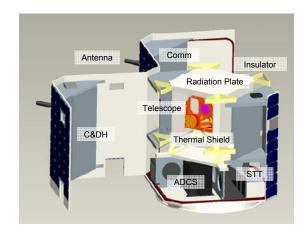
Figure 4-4: Inside Components Arrangement
