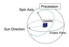
Figure 3-7: Spin Axis Precession
