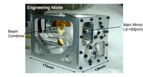
Figure 4-3: Telescope (Engineering Model)
