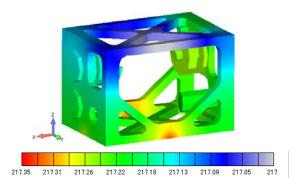
Figure 4-9: Telescope Part Precise Temperature Analysis
