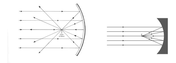
Figure 7: Light ray paths after reflection from a concave surface from Painter & Skewes (1950) and Oxenhorn (1970)
