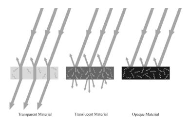
Figure 10: Representation of transparency, translucency, and opacity (Beauchamp, et al., 1958).
