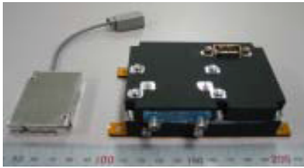
Fig.1: Left : Automobile-Navigation GPS Receiver CCA-370HJ, Right : Flight Model with RF Hybrid for INDEX Satellite
