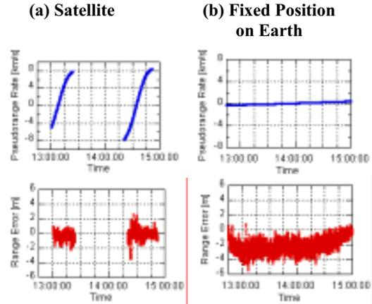
**Fig. 5: Pseudorange Rate and Range Error Based on GPS Simulation #1**
