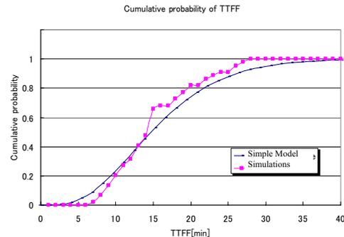
**Fig.3: Cumulative Probability of TTFB Based on GPS Simulation**
