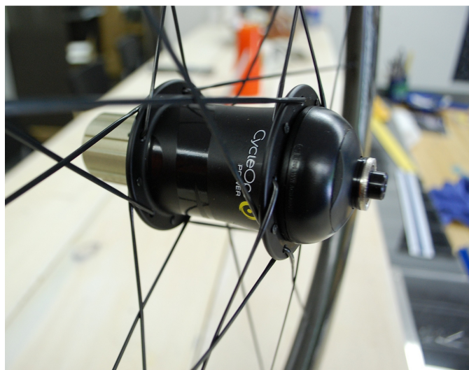
Figure 1. A CycleOps PowerTap power meter (3) in a bicycle wheel hub. Data are transmitted wirelessly to a bicycle computer
