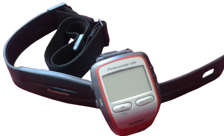
Figure 2. Garmin Forerunner 305. The device is a GPS wristwatch that wirelessly communicates with a heart rate monitor. Additional sensors can be paired as well.
