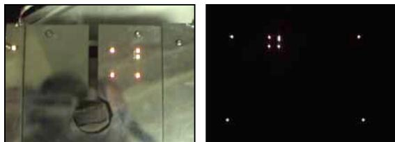
Figure 6: Bandit determines position by analyzing photographs of the Akoya LED array. Left: Short-range sorties use a small docking LED set. Right: Long-range sorties use large LED set.
