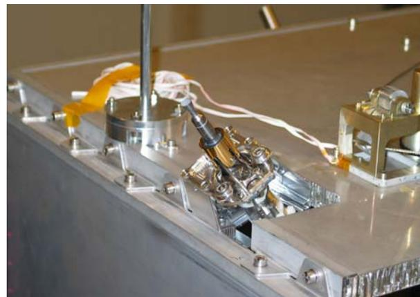
**Figure 3. The HPGP Thruster flight prototype during fit check on the STM spacecraft structure**
