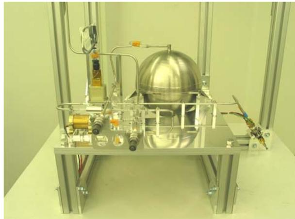
Figure 13. The HPGP Flight Propulsion System
