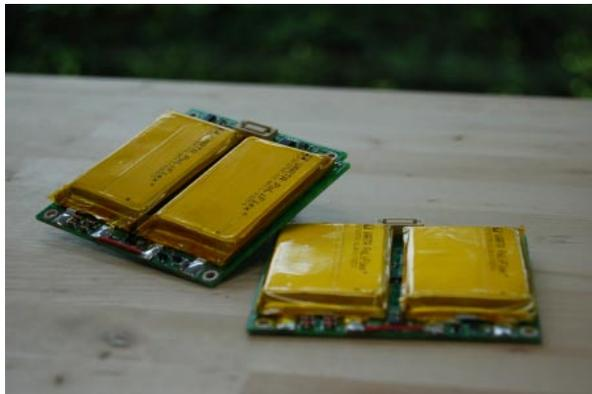
**Figure 15 Clyde Space CubeSat Lithium Polymer Battery**
