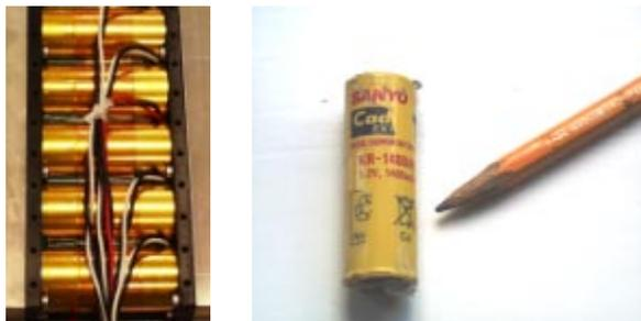
Figure 2 Example Palmsat Ni-Cd battery pack
