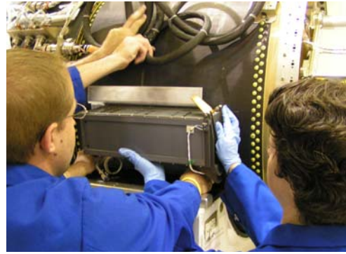
Figure 6: P-POD Fit Check
