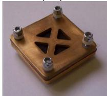
Figure 1: Finished Gold Plated Bio-Fuel Cell
