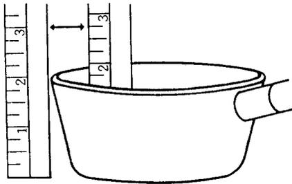
Figure 12. Checking Thickness of Cookware's Bottom.
