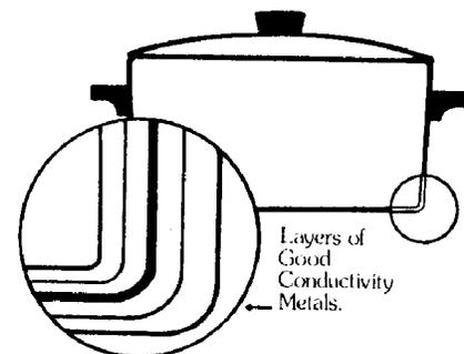
Figure 13. Metals Sandwiched Together.
