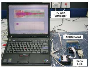
Figure 3: Actual Hardware-in-the-Loop Setup
