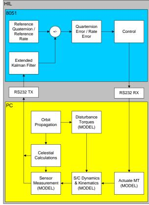
Figure 2: Block diagram of Hardware-in-the-Loop
