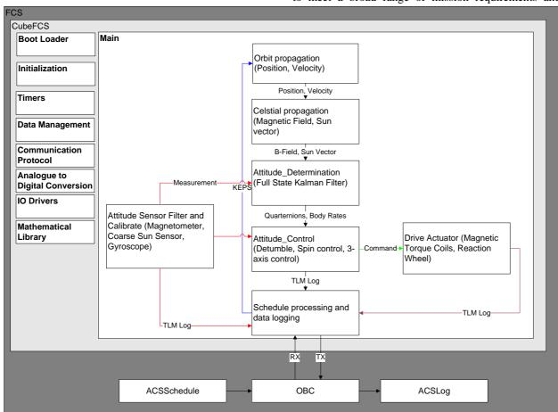
Figure 1: FCS Software Modules and Main Flow Diagram
