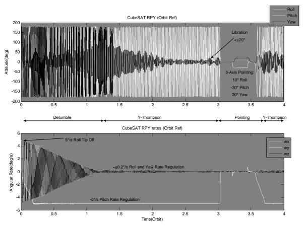
Figure 4: Emulation performance of CubeSat from detumbling to 3 axis pointing
