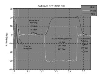
Figure 5: 3-axis pointing performance of CubeSat
