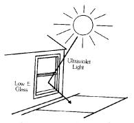
Figure 11. Low "E" Glazing Reflects Ultraviolet Light.
