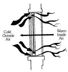
Figure 10. Heat Loss Through Windows.
