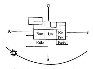
Figure 3. Placement of Most-Used Rooms.
