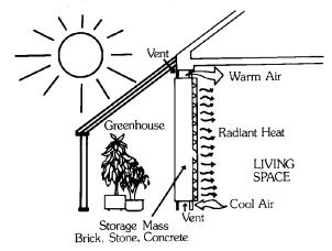
Figure 5. Thermal Storage Wall.
