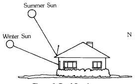
Figure 6. Roof Overhangs.
