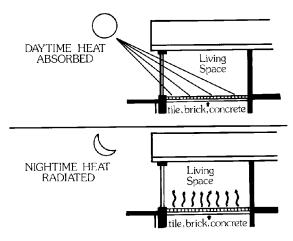
Figure 18. How Floor Materials Absorb and Radiate Heat.
