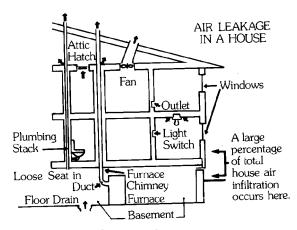
Figure 8. Air Leaks.
