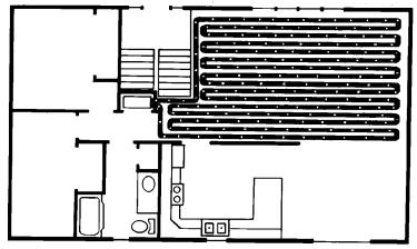
Figure 17. Floor Hydronic Heating System.
