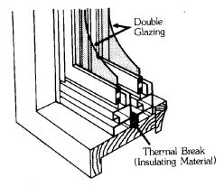
Figure 14. Window Thermal Break.
