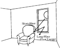
Figure 12. Low "E" Glazing Keeps Heat Inside.
